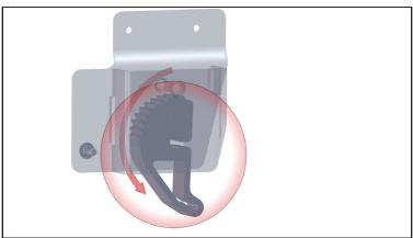
6. Make sure that you keep the rope brake cam locked in the position shown (the rope MUST follow the path of the arrow).
