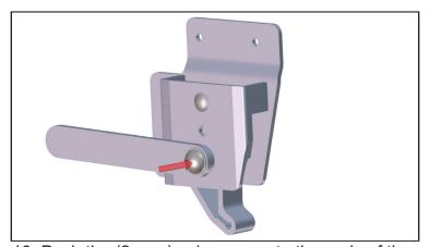
10. Push the (2 new) axle caps onto the ends of the square key with your thumb. DO NOT USE A HAMMER FOR THIS STEP. If you use a hammer you risk damaging the axle caps, and you will have to replace them. Once axle caps are on, make sure the Descent Control assembly functions properly before returning the CAGE to service.
