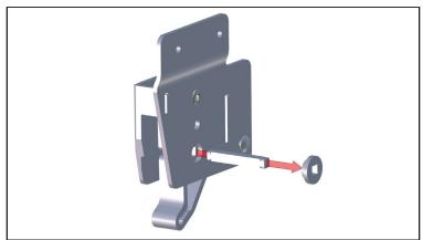
5. On the rear of the Descent Control housing, remove the square key bushings and square key (as shown in the illustration), then discard.
