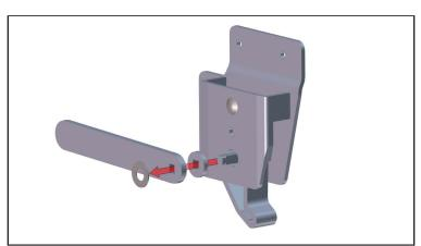
4. Once the (2) snap rings have been removed, remove the washer, handle, and square key bushing (as shown in the illustration), then discard.
