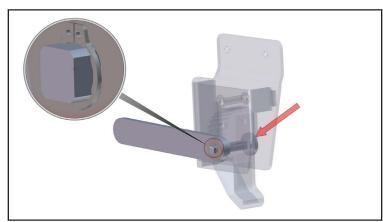
2. There are (2) snap rings located on the front and back of the Decent Control handle that are holding the square key in place.
