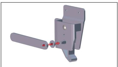
8. On the front of the Descent Control housing, insert the (new) square key bushing and the (new) handle (as shown in the illustration).
