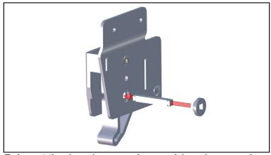
7. Insert the (new) square key and (new) square key bushing through the Descent Control housing and rope brake cam from the rear of the Descent Control housing.
