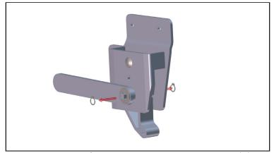
3. Using a pair of snap ring pliers, remove the (2) snap rings, then discard them.
