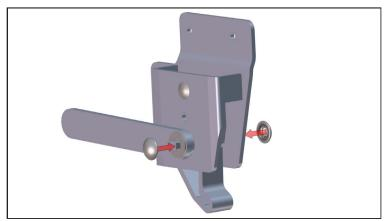
9. Line up and place the (2 new) axle caps on either end of the square key.
